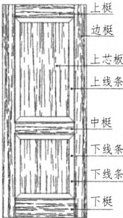
图1 拼装实木复合木门的门扇结构 Fig.1 Typical door leaf
