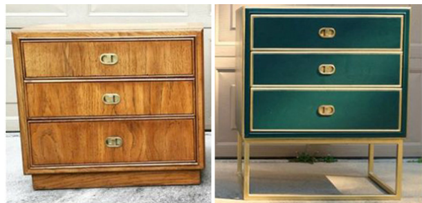
图7 旧木柜类家具增加部件复用方式 Fig.7 Reusing a used wooden cabinet by adding components
