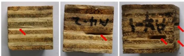
图2 白蚁沿着单板板层蛀蚀(箭头为白蚁蛀蚀孔) Fig.2 Termite damage along the veneer layer of plywood (arrows indicate termite damage holes)
