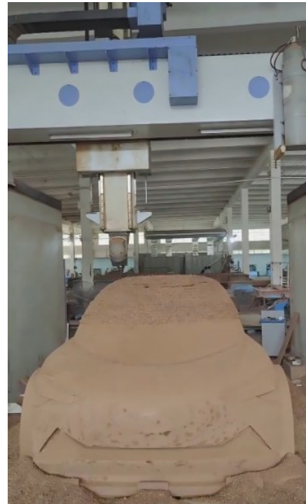
图10 五轴联动加工的木质汽车外观模型一体化成型加工 Fig.10 Integrated molding processing site for exterior model of wooden auto using five-axis coordinated machining
